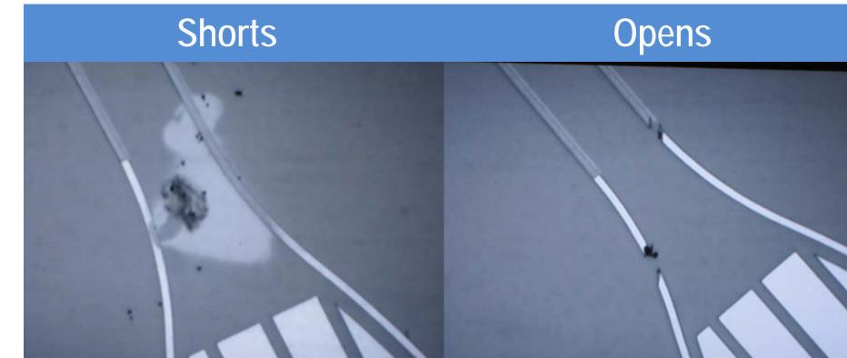
Two not so common defects are missing TES (Transition Edge Sensor) lines and bad overhang. Missing TES lines will cause the specific phonon sensor to malfunction. Bad overhang deteriorates signal transfer to tungsten sensors. Both defects result in unregistered phonons that directly hurt detector efficiency.
