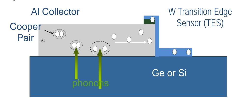
TES sensors held in equilibrium between normal and super conducting temperatures are highly sensitive to the small energy deposit from the quasiparticles.
