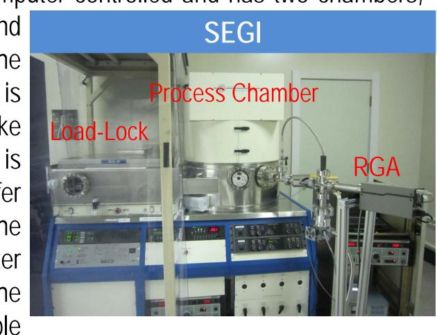
depositions with minimal personnel requirement. The advantage of two chambers is that the process chamber is always under vacuum. This minimizes contamination and speeds up the deposition process.
