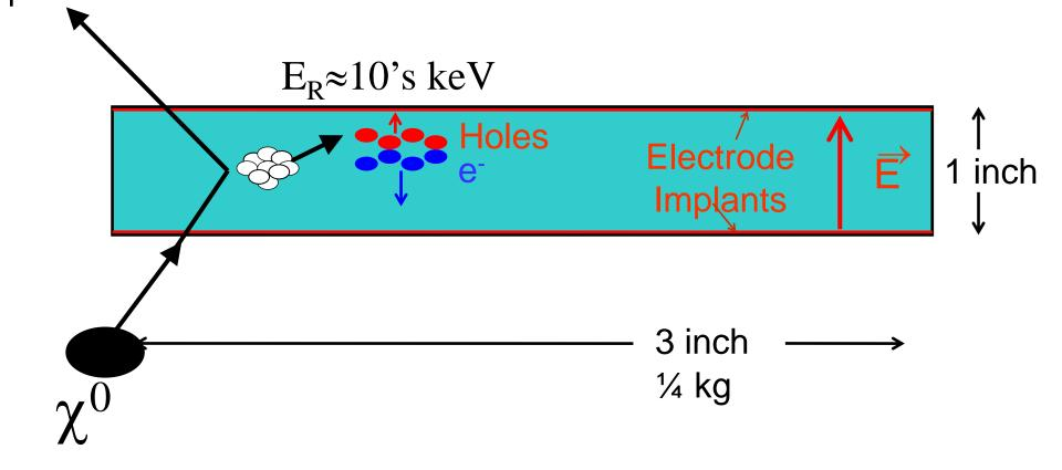
Generated phonons interact with cooper pairs in superconducting aluminum film deposited on both sides of germanium and create quasi-particles, which are then caught by a tungsten transition edge sensor.
