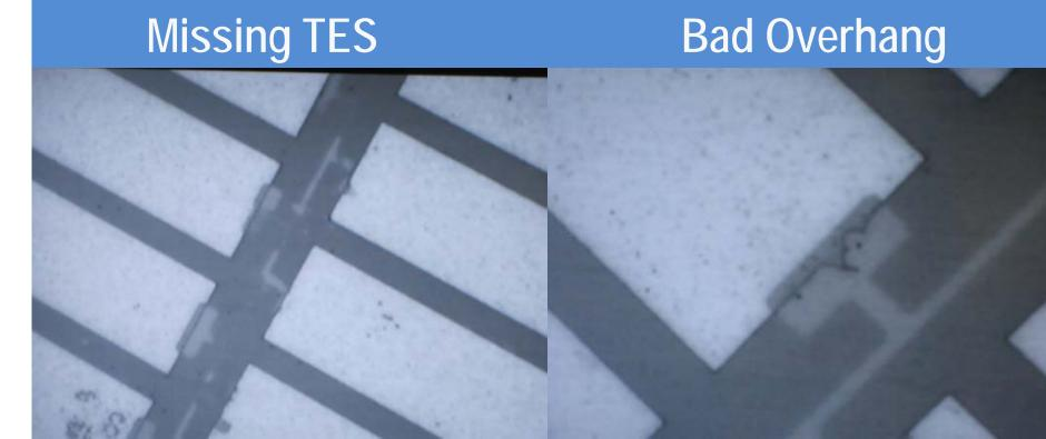
All substrates must be inspected to ensure none of these defects exist.
